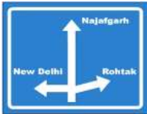
ADVANCE DIRECTION SIGN
