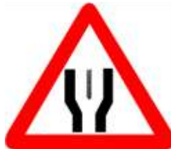
START OF DUAL CARRIAGEWAY
